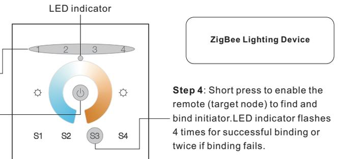
**Step 4:** Short press to enable the remote (target node) to find and bind initiator. LED indicator flashes 4 times for successful binding or twice if binding fails.
