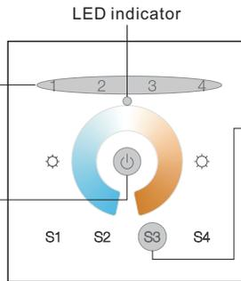
**Step 3:** Short press 5 times continuously to clear all bound lighting devices. LED indicator flashes 4 times for successful unbinding.
